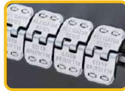
Staple type belt fastener as per ISO 14890 (RS62/125/187 Size, 17~35 KN/m, up to 6 mm Thick PVC Belt Joint)
