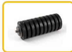
Impact Roller with Rubber Rings as per CEMA-B (114/140/165/190 mm OD, 76/89/114/139 mm Shell, up to 96 inch BW)
