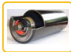
Conveyor Drum Pulley as per IS 8531 (~2200 mm Face W, 219~1000 mm Tube, 50~125 mm Shaft, up to 80 inch BW)
