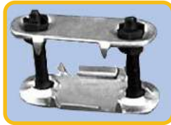
Solid Plate Conveyor Belt Fastener HAWK Type as per IS 10288 (1/1.5/2/2.5/3 inch Size, 150~560 P.I.W., up to 25 mm Thick Rubber Belt Joint)
