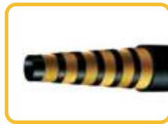
Water Blast High Pressure Jetting Hose per ISO 7751, Concrete Pump per EN 12001 (1000/85/100bar Pressure, 2.5:1/2:1 Safety, Spiral Wire/ Tire cord Ply, 12.5/19/63~125 mm bore ID)
